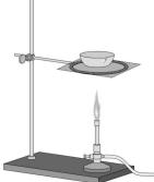
the ring and the evaporating dish containing the hydrate on the wire gauze. Use the diagram as a guide for your setup.
